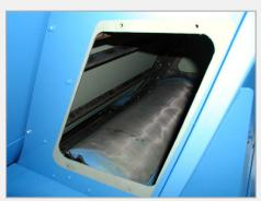
A single unit composed by one or several conveyors and a self-cleaning drum filter without disposable filtering fabric. Operation- costs saving and coolant life improvement. Ideal for machining centers, for all types of metal chips and coolants. Filtration degree down to 50 microns., flow following request.
