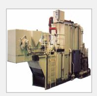
Omsat's FRD filter is a vacuum filter with flat endless not waste filtering belt, which stops during the suction time. Filtration is obtained by creating a mud cake.
