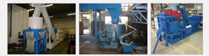
A centrifuge for each type of chips. Residual rate of humidity lower than 5 %. Rapid investment return.Any kind of metal chips. Implantation into a processing line of chips
